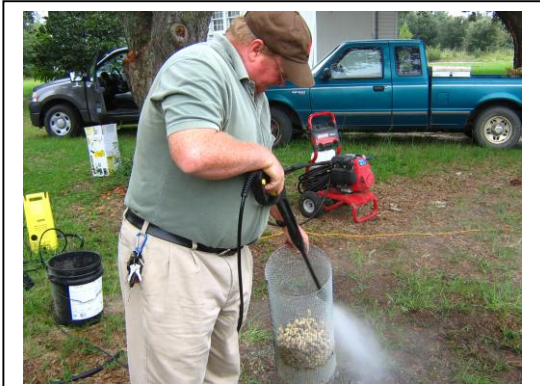
Use oscillating "turbo" nozzle, not high psi
