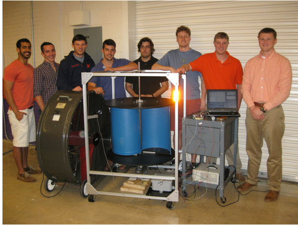
Vertical axis Savonius wind turbine for energy studies and real time controllable lift studies (target: ME 4440 lab, ME H4150)
