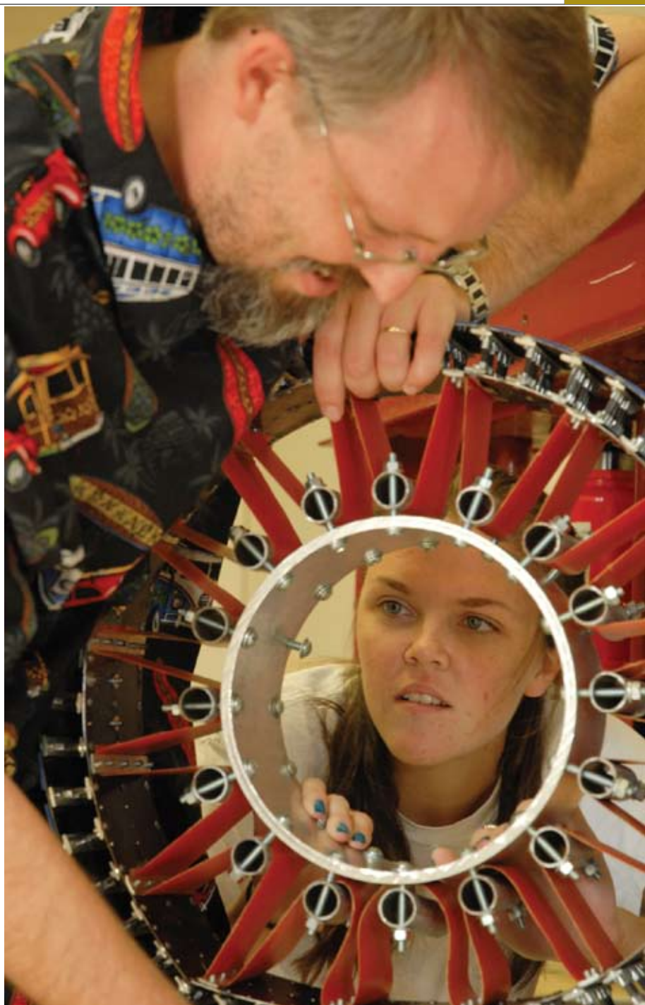
LUNAR TWEEL: Clemson University student-designed and built lunar tweel being inspected by Joshua D Summers and undergraduate student Samantha Thoe
