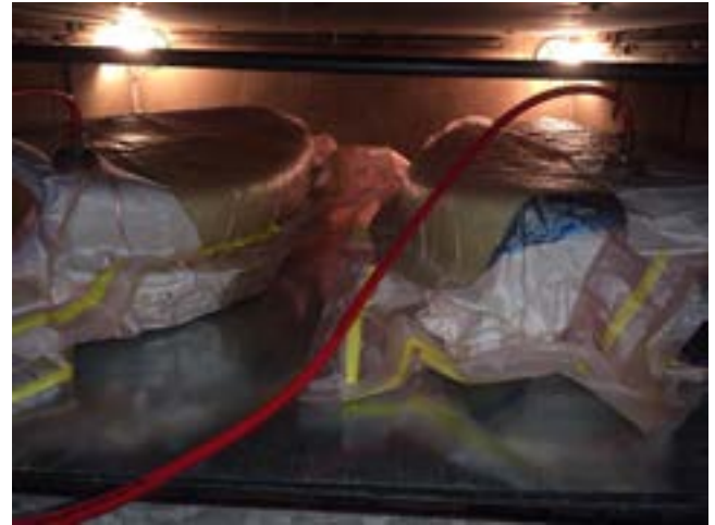
Tiger16's sidepods are put in our oven to cure, vacuum bagged using Airtech bagging materials!
