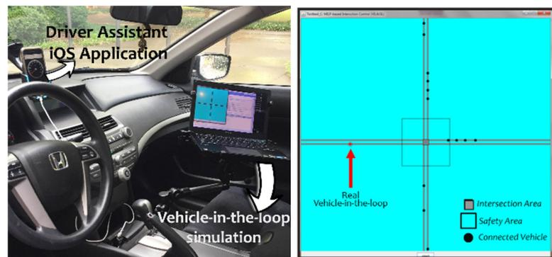
Figure 2: The real vehicle interact with hundreds of simulated vehicles in a microsimulation environment.
