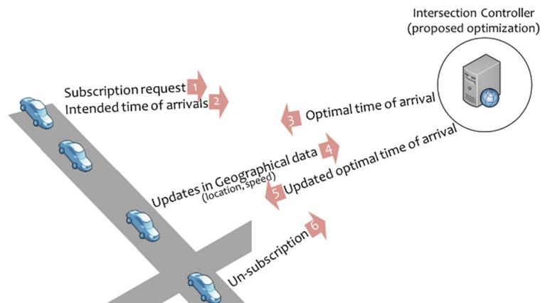
Figure 1: Path of data exchanged between the intersection controller and an approaching vehicle.
