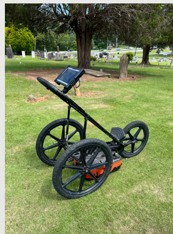
Ground-penetrating radar (GPR) surveying done on Old Stone Church's cemetery grounds in Clemson, SC. Photograph by Marquise Drayton.
